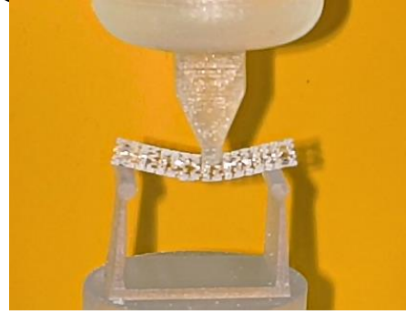
Real mechanical test setup for three point bend test (left); three point bend test simulation - boundary condition (right)
