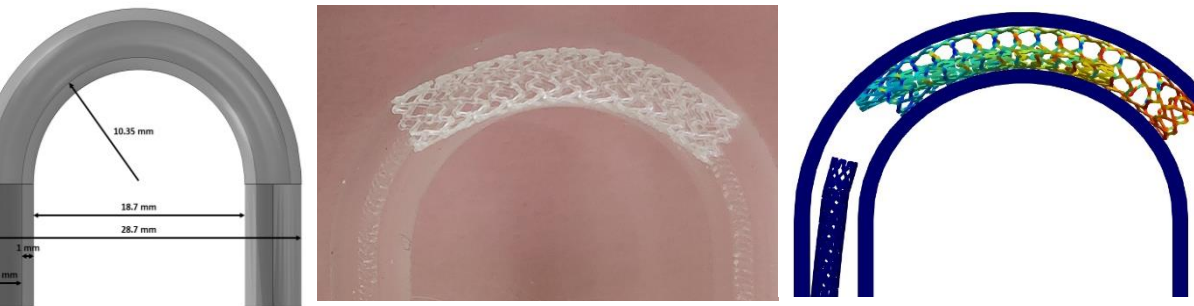
Flex test simulation - boundary condition (left) Real mechanical test setup for flex test (middle); Flex test simulation – results stress distribution (right)
